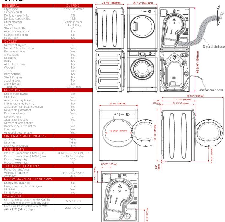
Stacked installation minimum air gap clearances: 6 1/4" top, 1/2" sides, 4" back, front 1/2"
