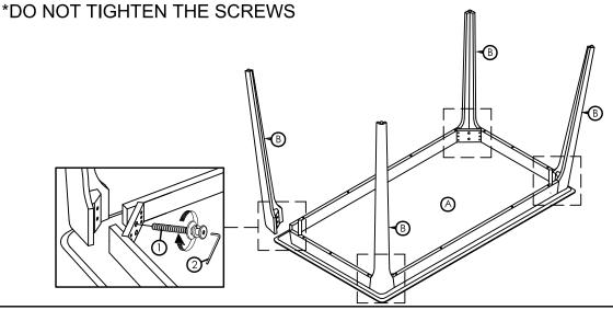
STEP 2: To level the table, place the table right side up on a flat surface and tighten the bolts with Allen Key (2).
