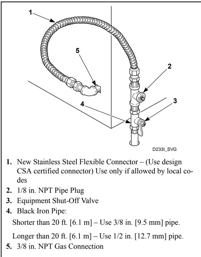
1. New Stainless Steel Flexible Connector – (Use design CSA certified connector) Use only if allowed by local codes
