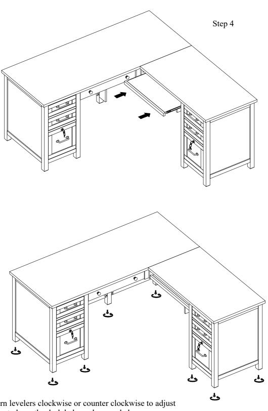
NOTE: turn levelers clockwise or counter clockwise to adjust the levelers to keep the desk balanced as needed.
