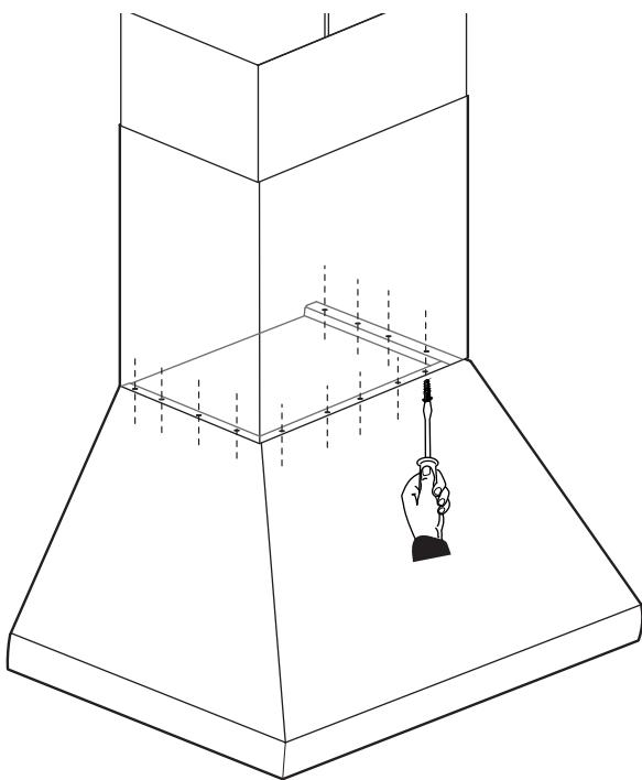
6. Carefully pull the top part of the extension upwards. Screw the left and right sides of the extension to the mounting bracket with the supplied stainless screws.
