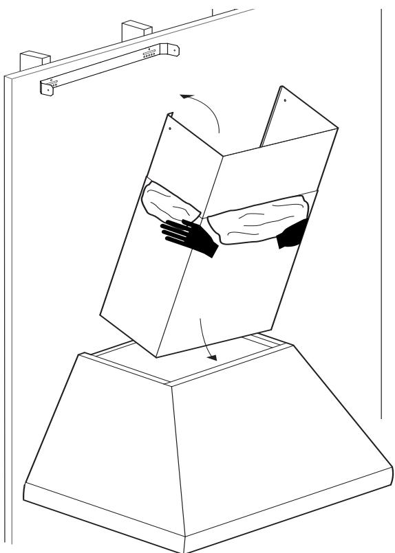
7. From inside of hood, screw the supplied 5/8" (16 mm) sheet metal screws through the holes on each side and along the front into bottom of the extension. Screw quantity is dependent on hood size.
