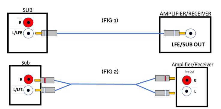
Stereo Pre-Out (FIG 2): If the amplifier/receiver is equipped with stereo (Right and Left) Pre Outputs then it can be connected to the subwoofer's right and left inputs with a stereo RCA wire. This is a common connection with integrated amplifiers.
