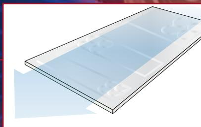
AIR IS BLOWN OVER A THIN ALUMINUM SHEET KNOWN AS A COLD PLATE
