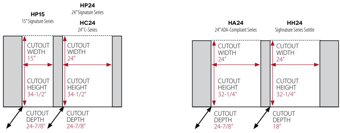
\* For all HP, HC, and HA models. To achieve 24" installation depth, install electrical connection in adjacent cabinetry. See spec sheets and installation instructions for install instructions.
