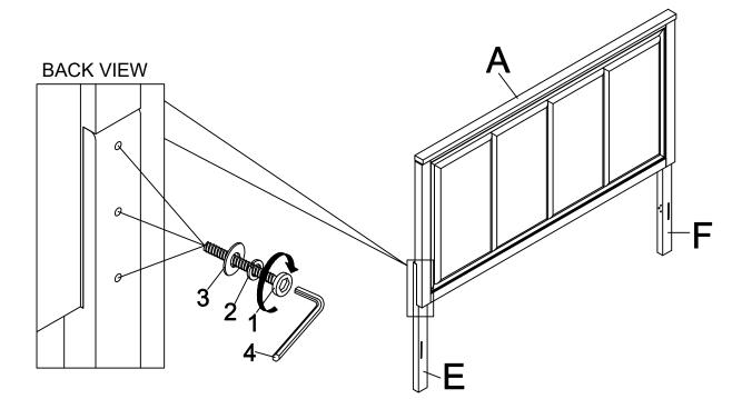
STEP 2 Assemble Headboard Crossbar (D) to HB legs (E) and (F) by using Allen Key (4) with hardware 1, 2, and 3.
