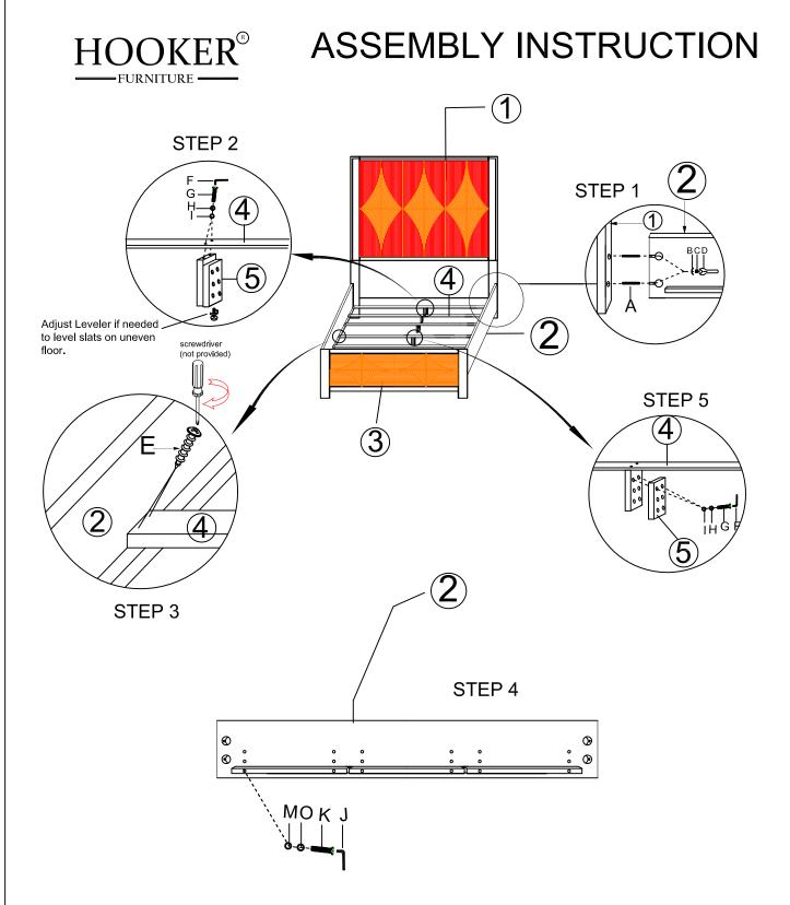
Note 1: You can change the height of slats (4) by adjusting the height of cleats on side rail (2) as shown in Step 4.
