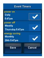
Once the Event Timers are adjusted, press the **Save** button. Pressing the **Cancel** button reverts to the remote's last saved setting.
