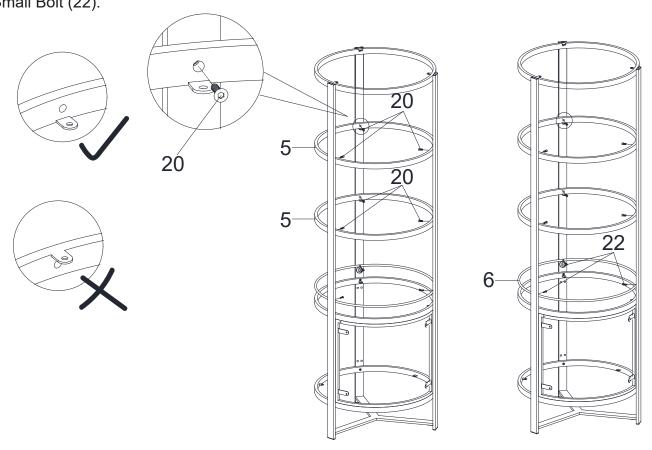
Step 6: Install Acrylic Side Panel (14) with Short Bolt (21).
