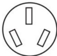
3-wire receptacle (10-50R)
