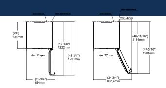
Allow door swing clearance at locations next to a wall. If the appliance is installed with the hinges next to a wall, the distance between the appliance and the wall must be at least  $1\frac{1}{2}$ " (40 mm). This is how far the handle protrudes when the door is open. The refrigerator door must open to a minimum of 90° to allow the crispers to open and the shelves to be removed. A 90° door limiter is available for this model.
