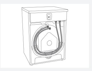
The water intake hose has to be fastened firmly enough for the hose to have a good seal.
