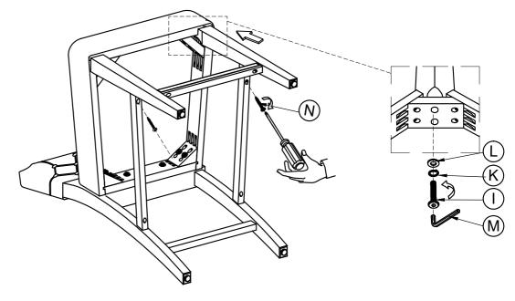
STEP 6: Using the Philips Head Screw driver to tighten all screws.
