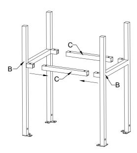
**Step 2.** Lay seat (A) down on a flat surface. Attach assmbled parts B, C to the seat (A) using bolts (D), washers (F), allen key (H) in vertical direction. Cross direction by using bolts (E), washers (F), allen key (H). NOTE: Do not fully tighten bolt until all bolts are in place.
