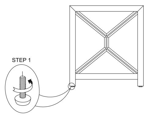
Adjust Leveler if needed to level case on uneven floor.
