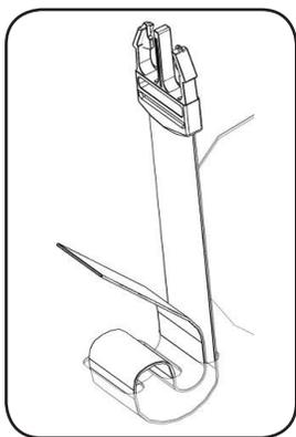
**Loop Strapping through slots in bottom shelf and secure over top of propane tank as illustrated**
