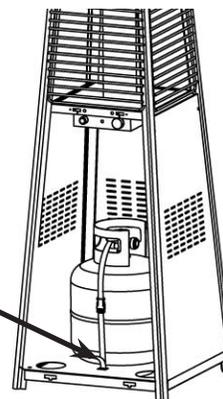
**Cylinder Connection:** Ensure the gas regulator hose is kink free. Remove the cap from the cylinder fuel valve. Insert the black QCC1 regulator nipple onto the QCC1 fuel valve. Hand tighten clockwise. Do not use tools. Leak test all joints prior to using the patio torch. A leak test must be performed annually and each time a cylinder is hooked up or if a part of the gas system is replaced.
