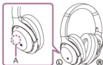
A: Location of the built-in antenna
