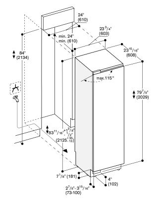
The door face dimensions are designed for a maximum gap of  $\%^{\prime\prime}$  (3 mm). See more details on page 252.
