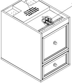
The above diagram shows a counter weight placed under the bottom of the fle cablnet. Do not remove this weight as it will greatly reduce the chance of tip over.
