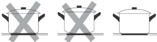
Make sure that the base of your pan is smooth, sits flat against the glass, and is the same size as the cooking zone. If you use smaller pot efficiency could be less than expected. Always center your pan on the cooking zone.
