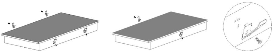
2. **Fix the cooktop to the cabinet:** Insert the cooktop into the kitchen cutout, as shown in the diagram below. The mounted clips on each side will secure your cooktop.
