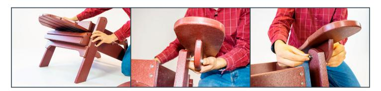
Lay the chair flat and open the front legs. Align the hole on the front side of the arm with the front leg. Insert a short bolt into the washer, arm and front leg. Slide on another washer and tighten a nut onto the bolt.
