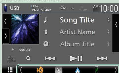
Display source selection icons by touching or flicking left or right on the source control screen, then select a playback source.
