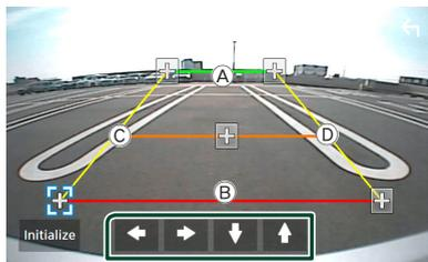
Make sure that lines (A) and (B) are horizontally parallel, and that lines (C) and (D) are of the same length.
