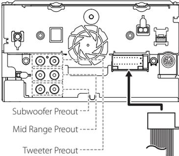
When connecting to an external amplifier, connect its ground wire to the car's chassis to avoid damaging the unit.
