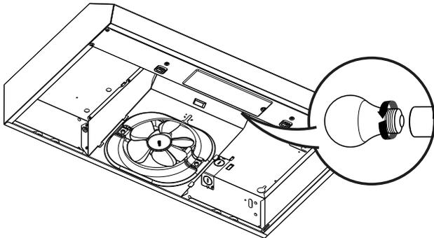
4. Screw a 120V, 9W maximum, LED light bulb with E26 base into the socket.
