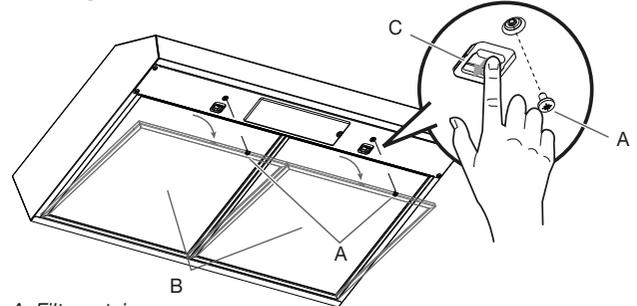
A. Filter retainer screws
