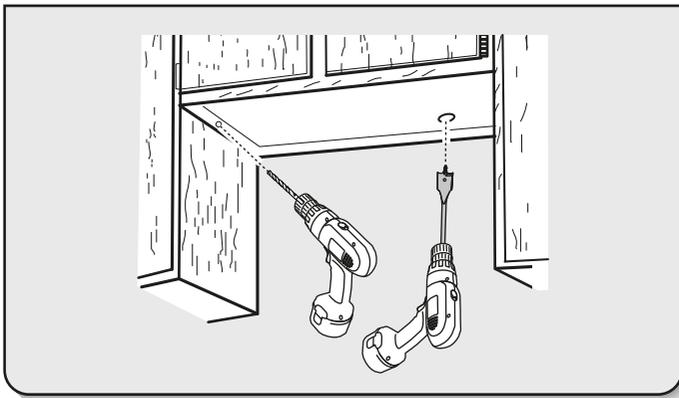
Using a 1¼" (3 cm) drill bit, drill the hole in the dot marked previously at the electrical strain relief.
