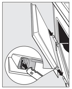
■ Hold both sides of the door securely and carefully fit it onto the brackets of the hinges.
