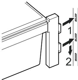
Insert the hooks of the rack into the openings of the clip-in strip at the desired height and push down.
