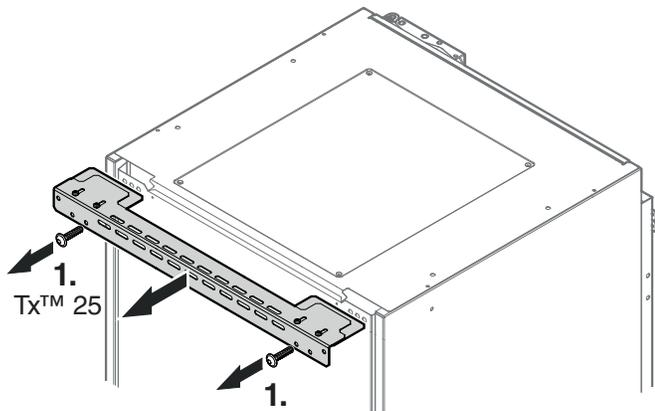
1. Remove the anti-tipping bracket. The screws are no longer needed.
