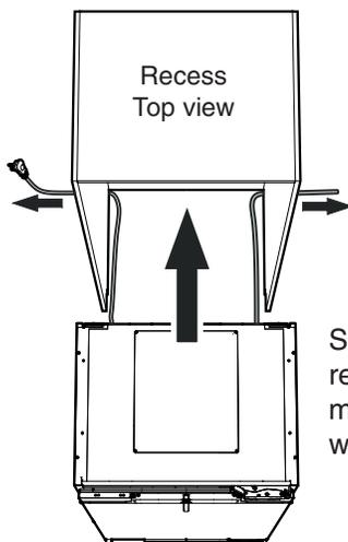
Slide the appliance into the recess. To avoid damage, move the power cord and the water line at once.
