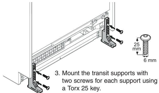
3. Mount the transit supports with two screws for each support using a Torx 25 key.
