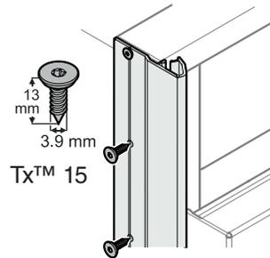
Apply the appliance cover strips to the left and right front edge of the appliance housing, align in height with the top profile and screw into place. The strip is transparent so the designed mounting holes on the appliance housing are visible.
