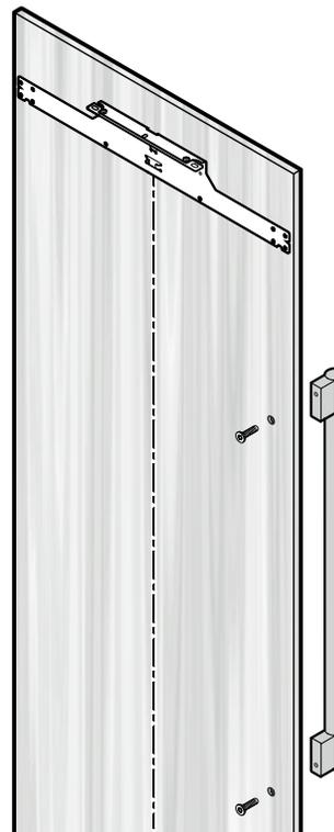
Only use countersunk screws for handle mounting.
