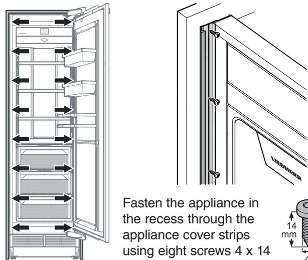
Fasten the appliance in the recess through the appliance cover strips using eight screws 4 x 14 for each side.
