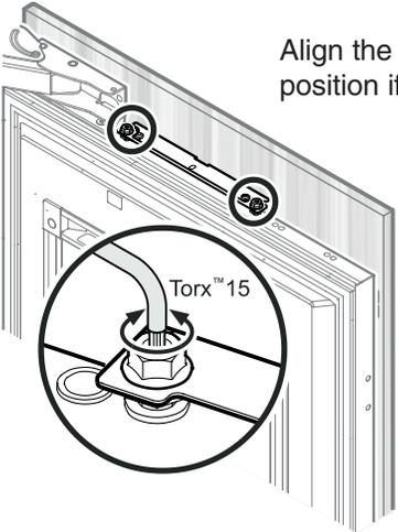
Align the panel in its vertical position if necessary.
