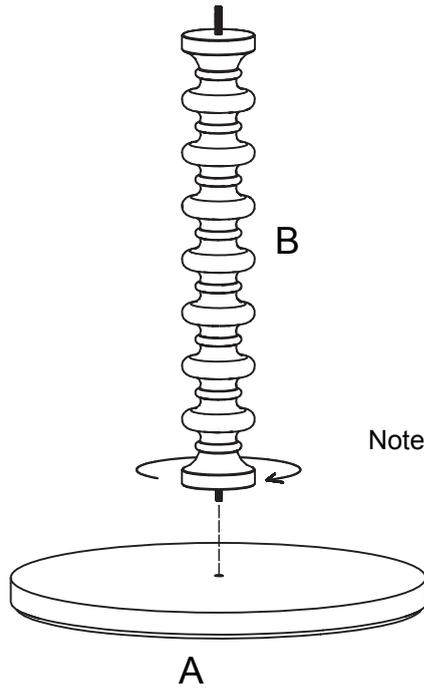
Note: The end of Post B with short exposed hardware is for connecting to Top A.
