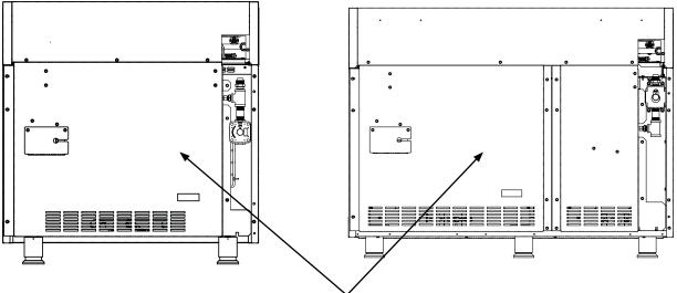
Remove rear panel to access infrared broiler orifice.
