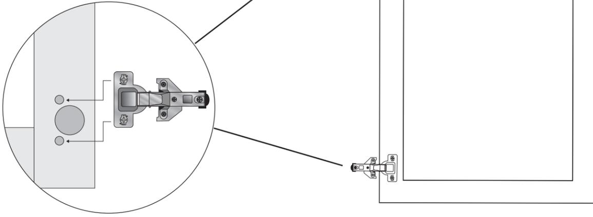
**Note: The hinge can be separated by pulling the black tab and pulling apart the hinge from the hinge base. Separated hinges snap back together.**
