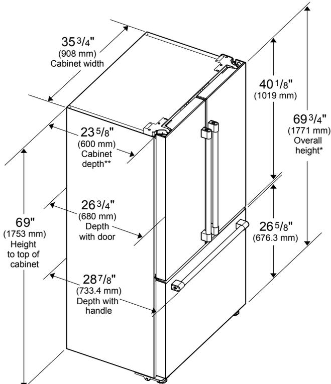
\*Add 1" (25.4 mm) with front leveling feet fully extended
