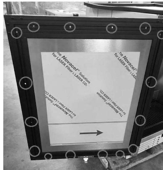
5. Loosely attached the four corners of the overlay panel with the door frame with #10 x 3/4" wood screws.
