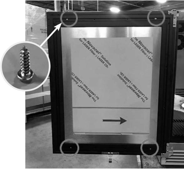
7. After alignment is satisfied, fasten down all screws through the screw holes.
