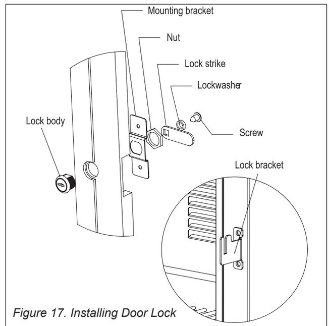
Figure 17. Installing Door Lock
