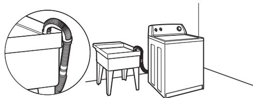
Minimum capacity: 20 gal (76 L). Top of laundry tub must be at least 39" (991 mm) above floor; install no higher than 96" (2.4 m) from bottom of washer.
