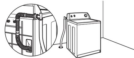
Minimum diameter for a wall or floor standpipe drain: 2" (51 mm). Minimum carry-away capacity: 17 gal (64L) per minute. Top of standpipe must be at least 39" (991 mm) high; install no higher than 96" (2.4 m) from bottom of washer. A sump pump system is required for higher installations.
