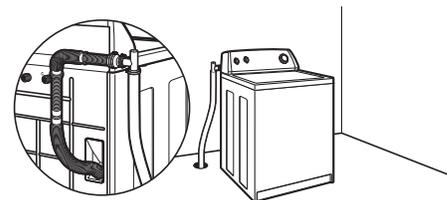
Floor drain systems require a Siphon Break Kit (Part No. 280129) and additional drain hose (Part No. 3357090). Minimum siphon break: 28" (711 mm) from bottom of washer. Additional hoses might be needed.
