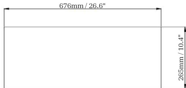
NOTE: Drill a hole in the cabinet measuring 676 x 265mm (26.6" x 10.4"). Make sure the distance between the edge of the hole and the front and rear edges of the cabinet is at least 35mm (1.4") to center the hood in the cabinet. The thickness of the cabinet should be limited to 15-25mm (0.6"-0.98") for best results.
