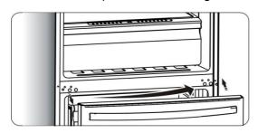
8. Remove screw hole cover (left) from the top left side of appliance and install it onto the top right side of refrigerator body.
