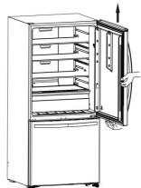
5. Loose screw (B) on the bottom of the fridge door and take down stop block (A), then install stop block (A) to the left side with screw (B).
