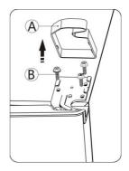
3. Remove the upper hinge (Please hold upper door by hand when installing). Keep it for future reference.
