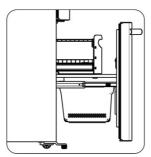
2. Take out the upper freezer drawer (A) by lifting it up from the rail system (B). Then push the rail system (B) back.
