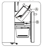
4. Remove the lower freezer drawer by lifting it up.
