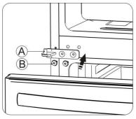
10. Close the freezer door. Refer to step 4, put the fridge door back on the other side, then close the fridge door and move it to an appropriate position.
