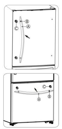
• When you reverse the fridge door, please move the handle (A), the screws (B) and the handle supports (C) to the right side. Move the screw hole covers (D) to the left side.
