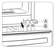
7. Change screw hole covers and screws on middle cover plate from left to right.
