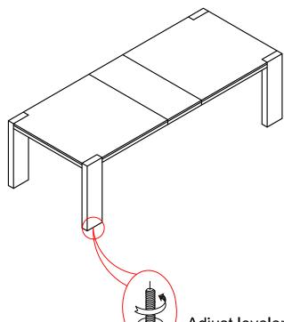
Adjust leveler if needed to level table on uneven floor.
