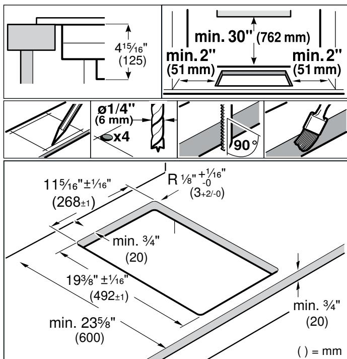
**Combining several Vario appliances:** Consider additional space requirement for the connecting strip VV 200 when making the cut-out. Appliances can also be installed in individual cut-outs, if a minimum clearance of 1 1/2" (40 mm) between the appliances is observed.
