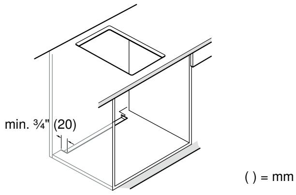
**Note:** If the appliance is installed in an island unit or another installation that is not described here, you must ensure that the cooktop is sufficiently ventilated.
