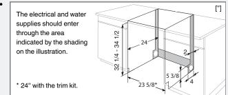
Make sure the area on which the dishwasher is to be installed is firm. Adjust the adjustable feet so that the dishwasher is level. Tighten the lock nuts.
