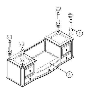
Step 1: Lay the vanity box (A) face down on a piece of cloth or carpet to prevent finish from scratching. Assemble the vanity box (A) with leg (B), tighten at this time.
