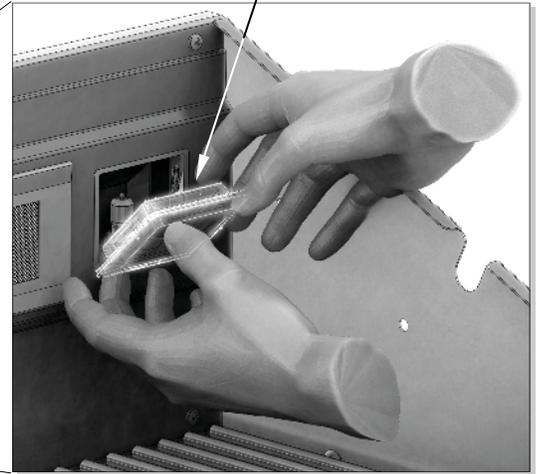
The light cover is supported by a spring mechanism on the light fixture. Simply pry open the light cover from the left or right side by hand only.
