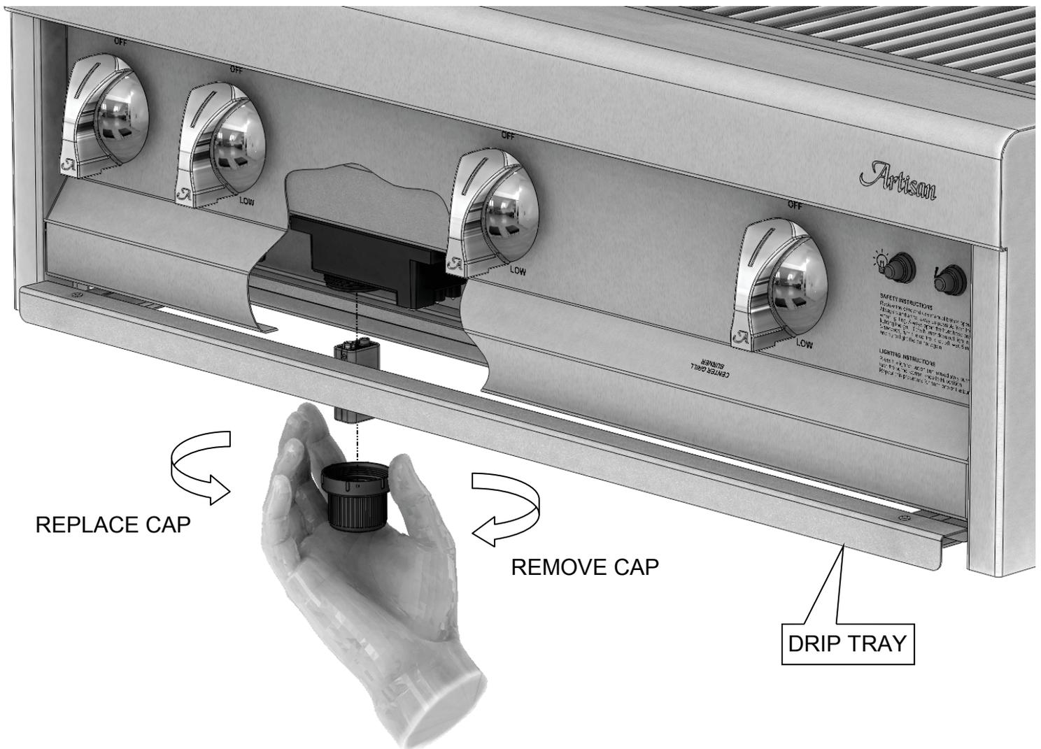
To insert or replace the battery which powers the igniters:
