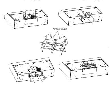
7. 10"x3 1/4" horizontal ducting: Remove the back cover (fig.1) and then fix the ducting (fig.2).
