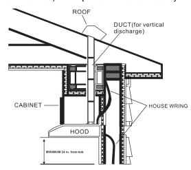
Determine whether the hood discharge vertically round (6in.) For vertically run ductwork between the hood location and the roof cap or wall cap. For the best result, use a minimum number of transitions and elbows.
