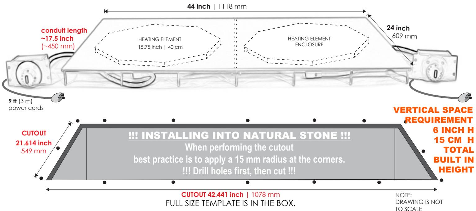
▶▶ **Control Box MUST be firmly fastened to a NON-MOVING surface. Power Cords and Conduits must be secured.**
