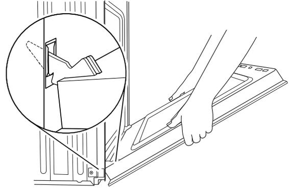
**IMPORTANT:** Do not close the door at this step or damage may occur to the door hinge.
