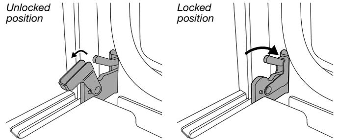
7. After the door hinges have been locked, gently swing the door upward to close. The door should not be forced closed.
