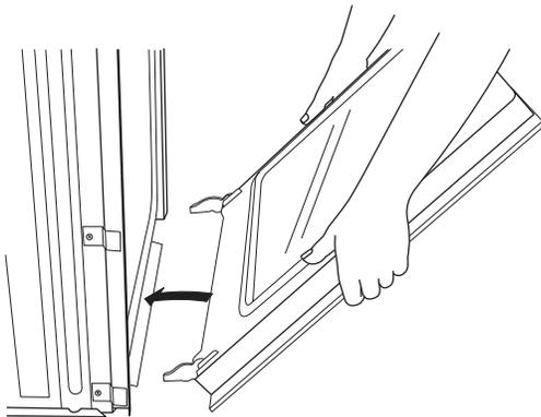
4. Make sure the door hinge notch is engaged on the bottom of the oven cavity slot.
