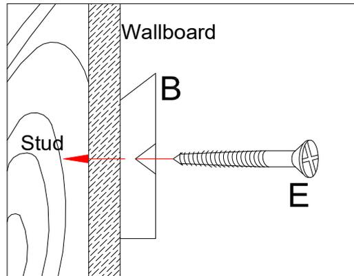
**Step 6: If hole locations do not align with stud in wall, install the EZ Anchor(F) in to drywall by tapping it in to the predrilled pilot holes up to the thread, and then screwing the EZ Anchor in to the drywall. Attach Cleat (B) using wood screw (E) to EZ Anchors. NOTE: Cleat could be secured using combination of Studs and EZ Anchors.**
