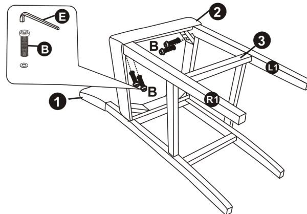
Put L1 and R1 legs in the holes. Then put 3 in the holes. Put the screws in the holes, tight the screws, but not too tight, 90% is ok.
