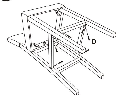
Put the screws in the holes, tight the screws, but not too tight, 90% is ok.
