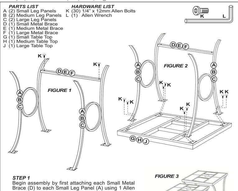
Bolt (K) per each end. Do not fully tighten bolts. See Figure 1.
