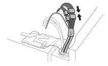
Push the water supply lines into the hole on the top case and pull them through the backplate.
