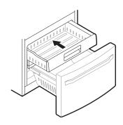
Replace the ice bin(s) in the drawer. Insert the Durabase basket in the rail assembly.
