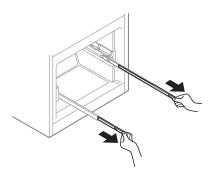
Grasp the drawer on each side and hook the drawer supports into the rail tabs located on both sides.
