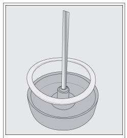
If necessary, you can remove the connecting piece and seal from the milk flask lid. Once you have removed the stainless steel tube, the connecting piece is easy to push out from the inside of the lid. Clean the individual components in a dishwasher.
