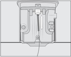
Push the cleaning brush a maximum of 3/8" (1 cm) into the steam jet.
