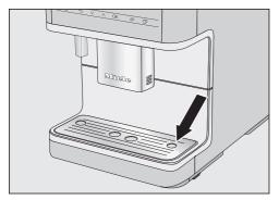
Replace the drip tray cover. Make sure that the drip tray cover is correctly installed (see illustration).
