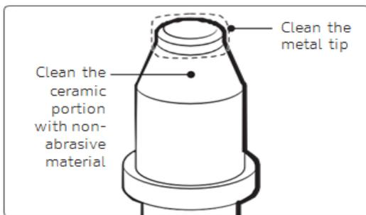
Do not cook while you clean the cooktop. Ensure the white ceramic electrodes are clean and dry. Clean the metal with a soft cloth. Do not clean the igniters with water.
