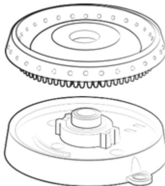
1. Put the burner heads on the burner bases. The bottom of the head fits inside the top of the base.
