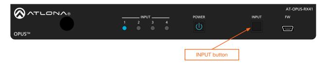
After the **INPUT** button is pressed, the INPUT LED indicator will advance to the next input, in sequence. In this example, **INPUT 2** is the active input and is indicated by the **INPUT 2** LED indicator on the front panel.
